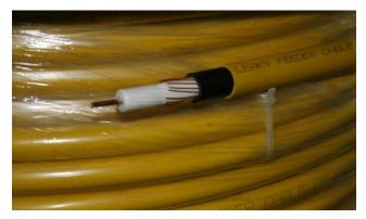
This is a communications system that is used in underground mining and other tunnel environments. The leaky feeder communication system consists of a coaxial cable that runs along tunnels or underground mines which emits and receives radio waves thereby functioning as an extended antenna.
