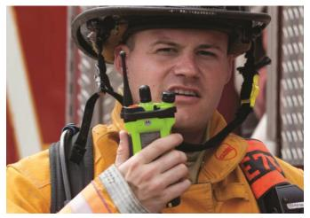
An Intrinsically safe portable radio that has been designed to the correct standard can provide all the features and performance of a non-Intrinsically-Safe model.
